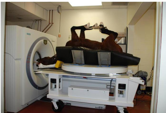
The system shown uses a direct drive lead screw (no gear head) to position a horse within the CAT scan machine for diagnosis and treatment. The PVIA control system was able to handle empty table to a 3000 pound horse and speeds from 0.1mm/second up to 4cm/second all with the same tuning with a 1 stack 34 frame motor.
