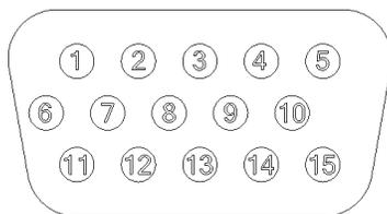
N2: V+, N3: Controller V+ and Drive Enable rated +12.5 to +48 VDC.
