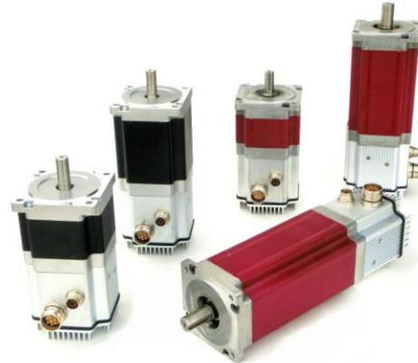
are also included. Communication via CANopen and RS-485 serial, which may be operated simultaneously. The driver is rated to 20A continuous per phase, 12.5v to 72v. The Processor section is designed for use at +12.5 to +48 VDC. Rated IP65 except front shaft. The QCI-X34HC family may be ordered with front shaft seals installed. Contact Factory.
