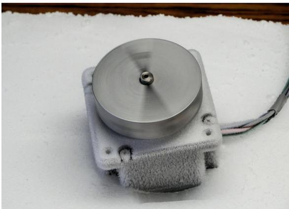
The Mosolver works over a wide range of temperatures. The picture shows a 23 frame Mosolver operating in a block of Dry Ice. For high temperatures, the Mosolver should be able to match the ratings of the motor as well.
