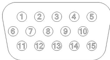
S2: V+, S3: Controller V+ and Drive Enable rated +12.5 to +48 VDC. All Power connections must be externally fused. See data sheet for details.
