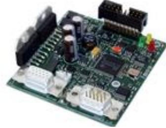
Power, communications, and I/O are accessed through a single DB15 high density interface connector. The interface includes 7 I/O, which support LVTTTL. 4 of the I/O also support analog signals. DMX is available with the D option. CANopen is available as the J option
