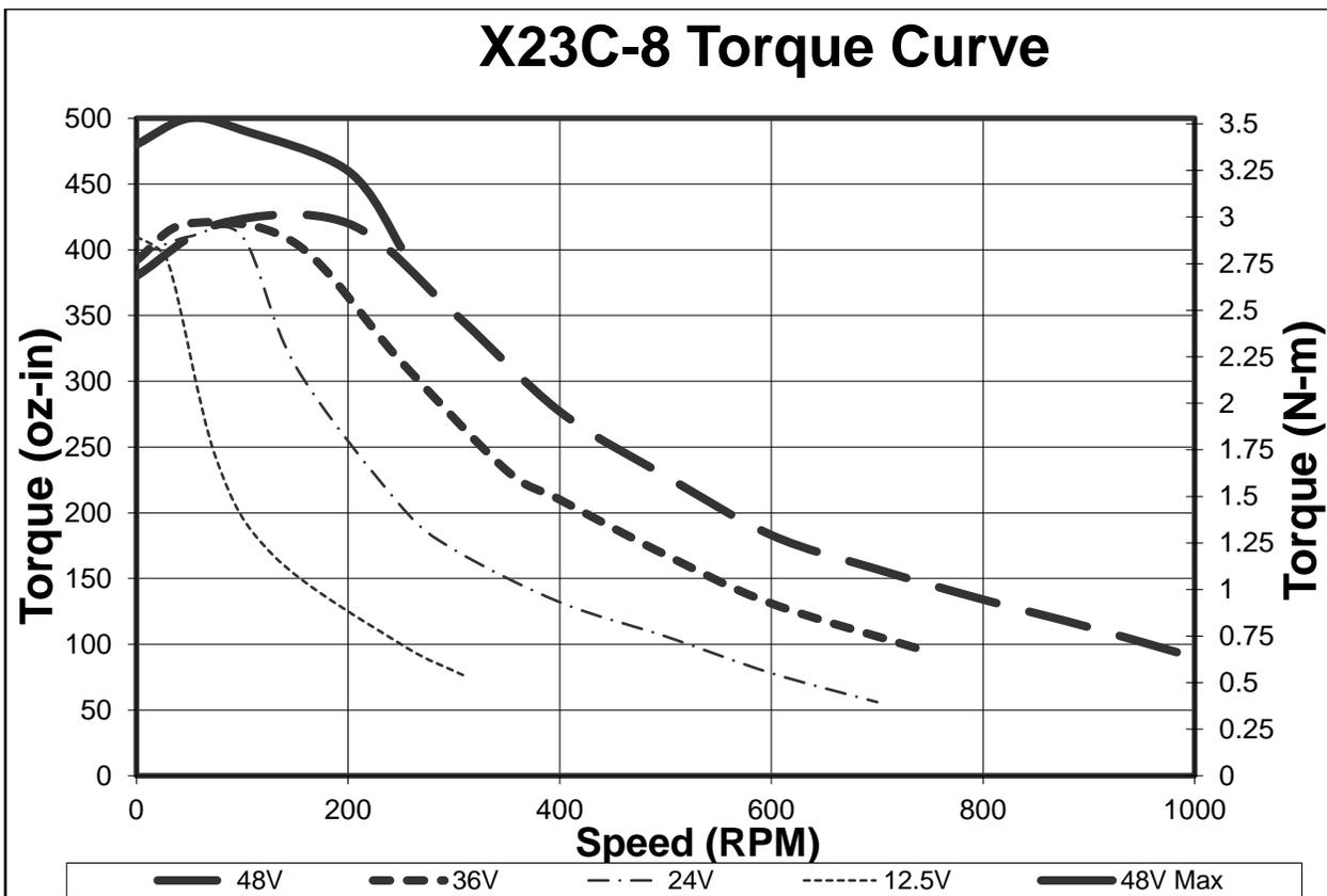
\*\*All Torque Curves in Catalog taken without shaft seal in place.
