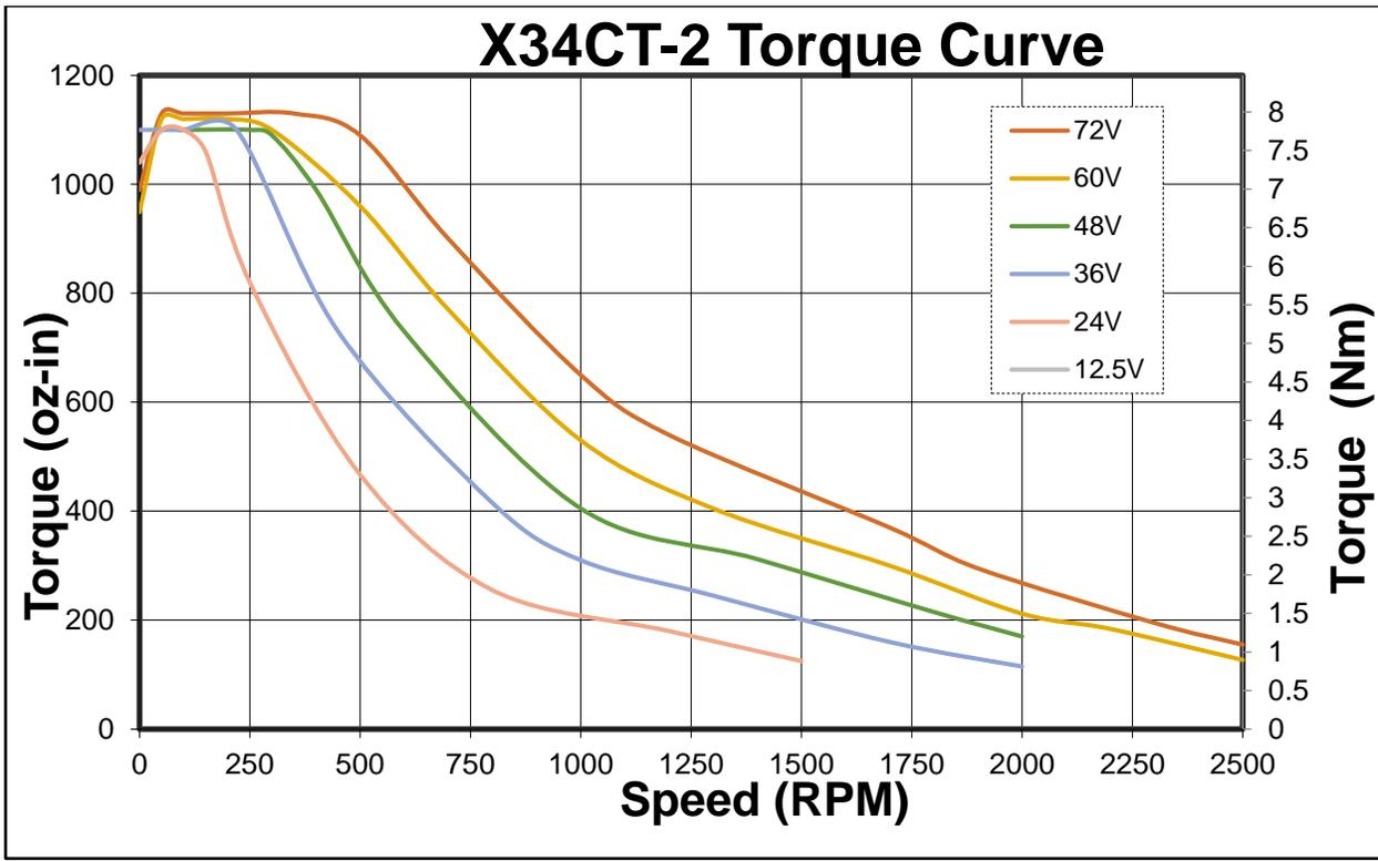
Note: All torque curves taken with 2' power cable; voltage measured entering power cable.
