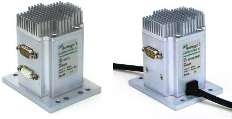
Power, communications, and I/O are accessed through a single DB15 high density interface connector. The interface includes 7 I/O, all of which support both LVTTTL and analog signals, and one of which also supports 0 to 10v analog. A hardware drive enable is available as a factory option (Special order). All 7 I/O also have soft configurable pull-up/pull-down resistors, which may also be disabled, for more flexibility
