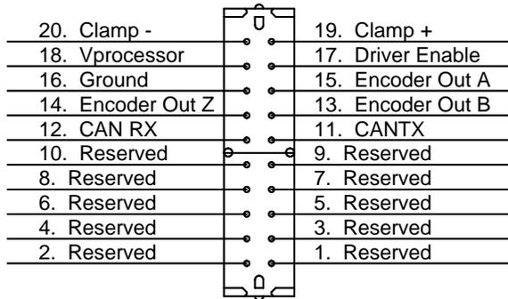
**Driver enable:** By default, the SilverDust IG comes with a jumper between pin 17 & 19 to automatically enable the driver. If user applications require a separate hardware drive enable, then use pin 16 and 17 to enable/disable motor driver.
