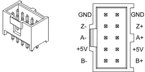
Encoder jumper block selects either single ended or differential encoder inputs. Single ended use the A+, B+, Z+ connections. These come jumpered for differential from the Factory.
